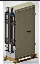
Close the doors to check alignment. Fully tighten the bolts (to 16 Nm) and install the cable bar (optional) at the lower end of the assembly. 5
