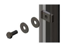
Fixings into Unistrut Channel (detail for info)
