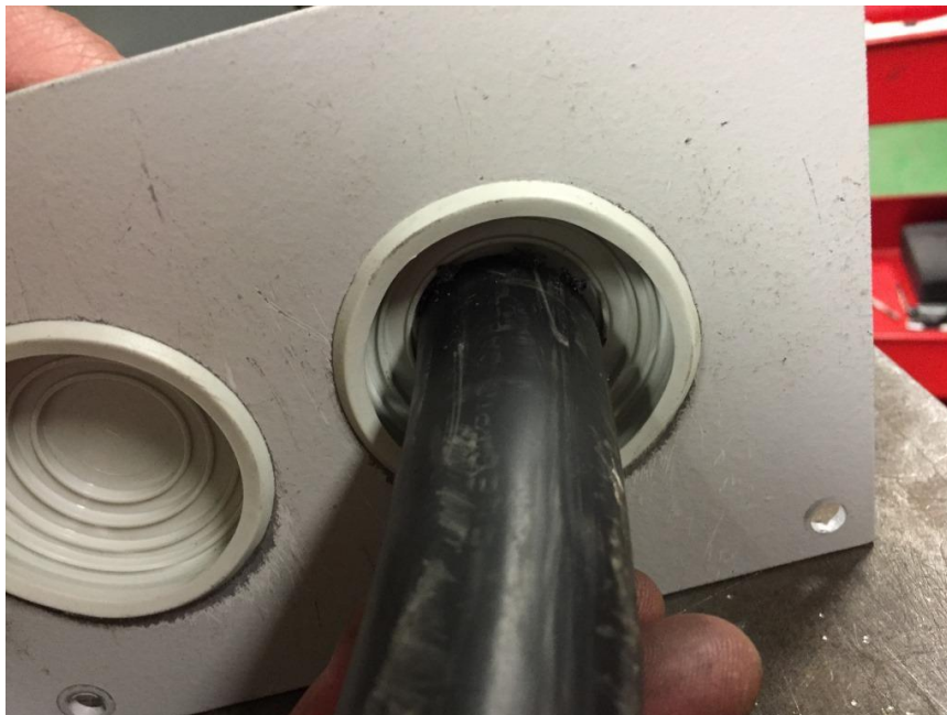
Figure 21: Membrane Gland Cable Sealing.
