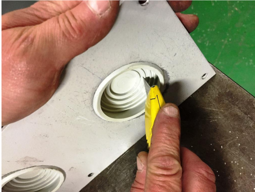
Figure 20: Cutting the Membrane Gland.
