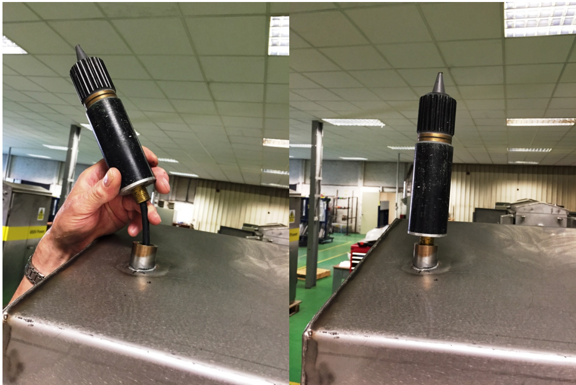
Figure 8: Installation of Precipitation Sensor
