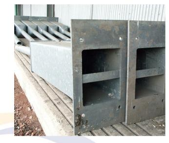
The Post 75 is manufactured from hot dipped galvanised mild steel and is designed to MCX 0174 to meet the highways agency specification MCE 1109 for the mounting of signal frames, electronic surveillance and meteorological equipment.
