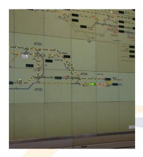
Mimic diagrams, in a variety of formats, have been manufactured by HWE Ltd for many years, with the premier style being the Domino <sup>®</sup> type. The original design of the Domino <sup>®</sup> style mimic was tailored to suit the railway industry, which required an easily modified system, that at the same time would be capable of maintaining safety at the highest level combined with a long operational life.
