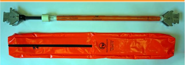
The Integrated Treadle Gauge eliminates the need for various measuring tools as previously required.
