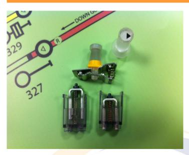
The Henry Williams Domino ® typesystem has been in existance since the 1950's many of which are still in service today, one of the areas of concern on older panels is the pushbutton spings and contacts, we have pulled together a pushbutton spares kits which can be installed into your existing top units extending the life of the panel.
